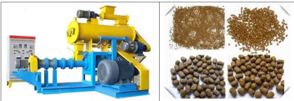
Figure 12: Photos of the fish feed pelletization machine and different classes of the fish feed pellets
