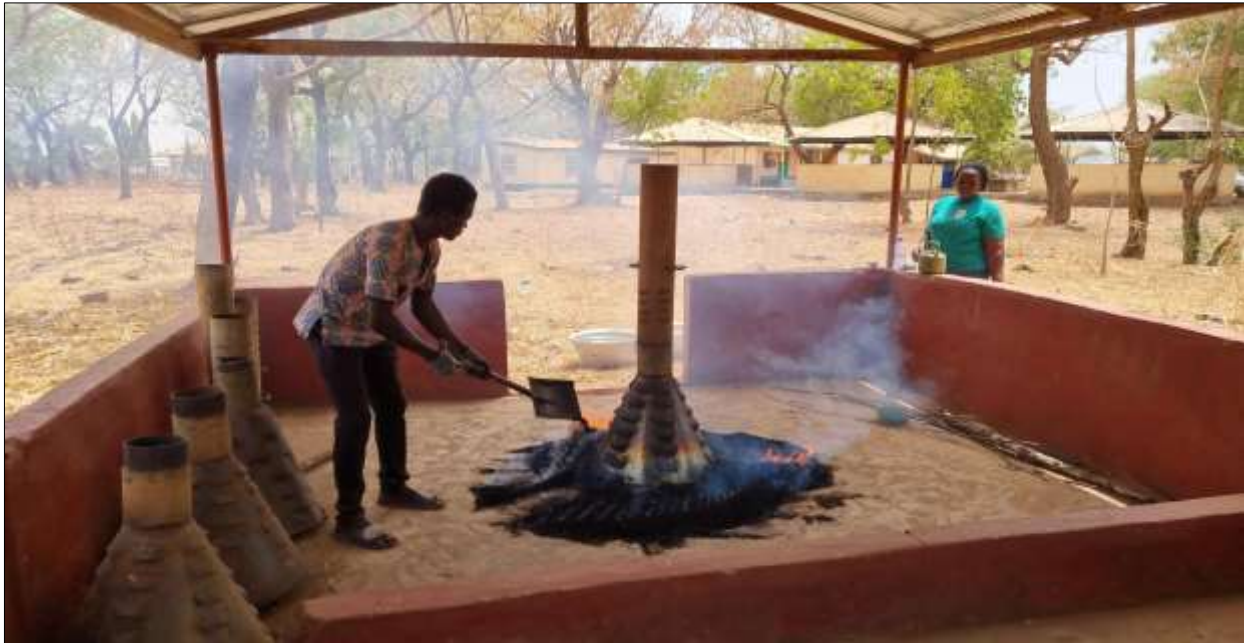
Figure 1: Photos of the Brazilian Kiln employed to produce high-quality biochar in Ghana
