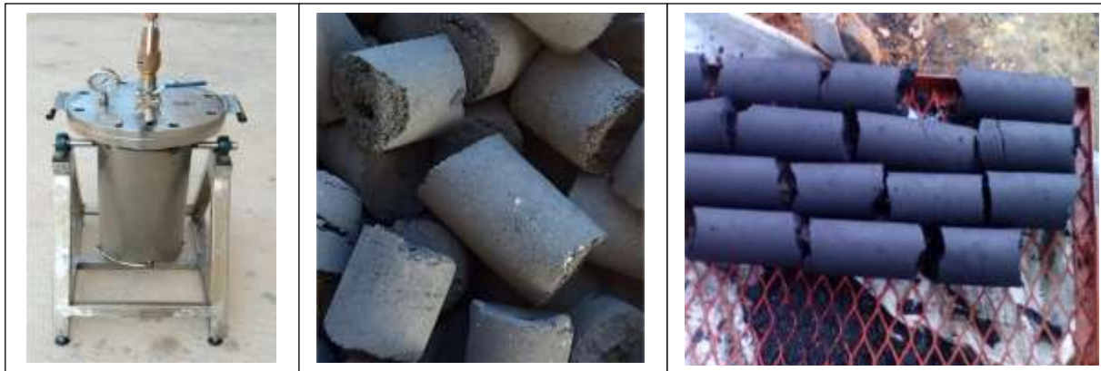
Figure 5: Photos of the new HTC device and high-quality biochar briquettes produced in Senegal
