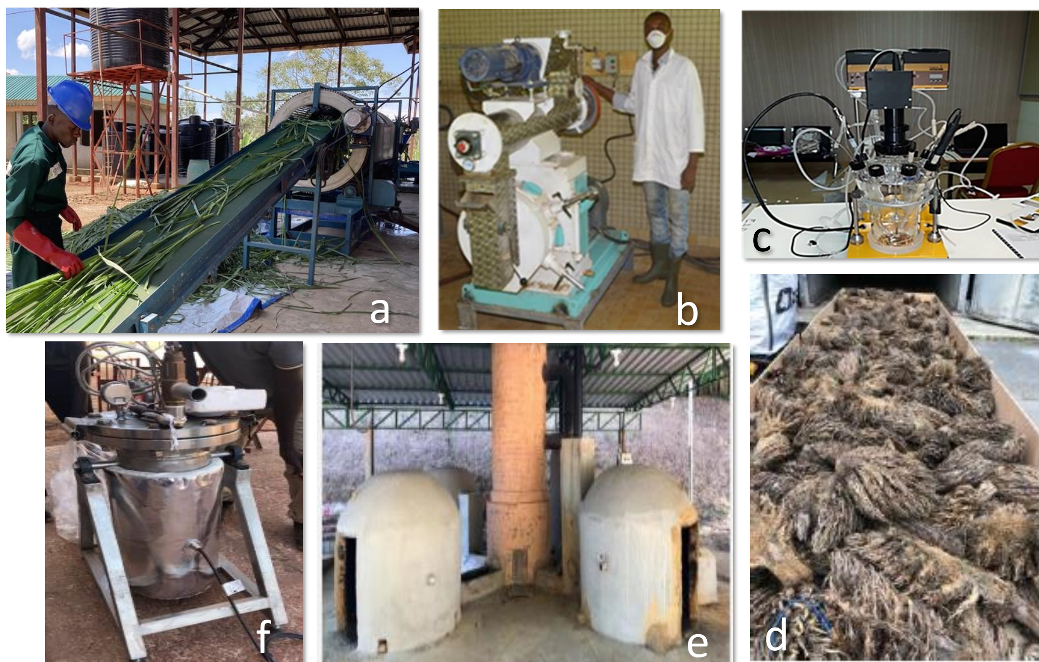
Figures: a) Biorefinery technology, KRC; b) pelletizing technology, INP-HB; c) 5L biofermentor for bioplastic production, INP-HB; d) empty palm fruit from UASZ being processed for biocomposite production; e) pyrolysis kiln model being constructed by SavaNet and INP-HB; f) hydrothermal carbonization equipment, UASZ
