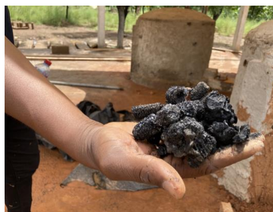
Figure 7: Biochar prepared from Maize cobs using the Brazilian kiln in Ghana
