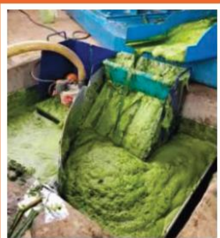
Liquid Whey from the Green Biorefinery for piglet feeds
